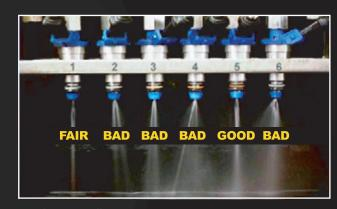
Professional off-vehicle diagnosis, testing and cleaning is the ONLY way to guarantee that your injectors are functioning efficiently and at their maximum performance.
